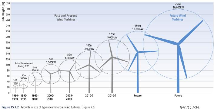
Figure TS.7.2 Growth in size of typical commercial wind turbines. [Figure 7.6]
